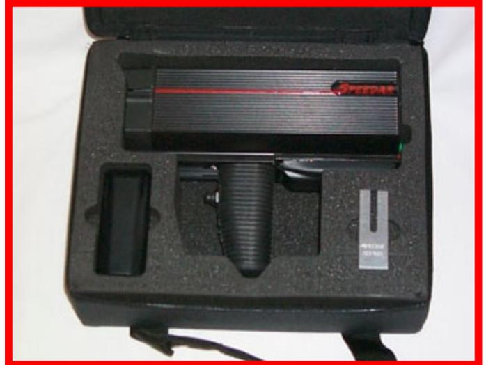
Cost of ownership is another factor. Lasers must be treated with considerably more care than radar guns. If the optics of a laser are disturbed through rough handling or impact damage (being dropped in other words) then the repair costs are going to be high and the time it is out of service may be long bearing in mind that it will almost certainly have to be returned to the manufacturers in the USA for repair. Of course you may be lucky enough to be loaned a replacement unit whilst it is away!
